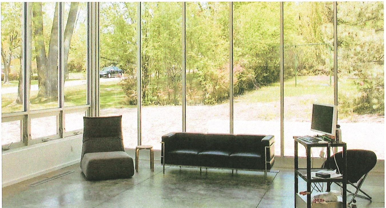
- The double height living room window faces north, bringing daylight deep into the space while avoiding direct sun.
