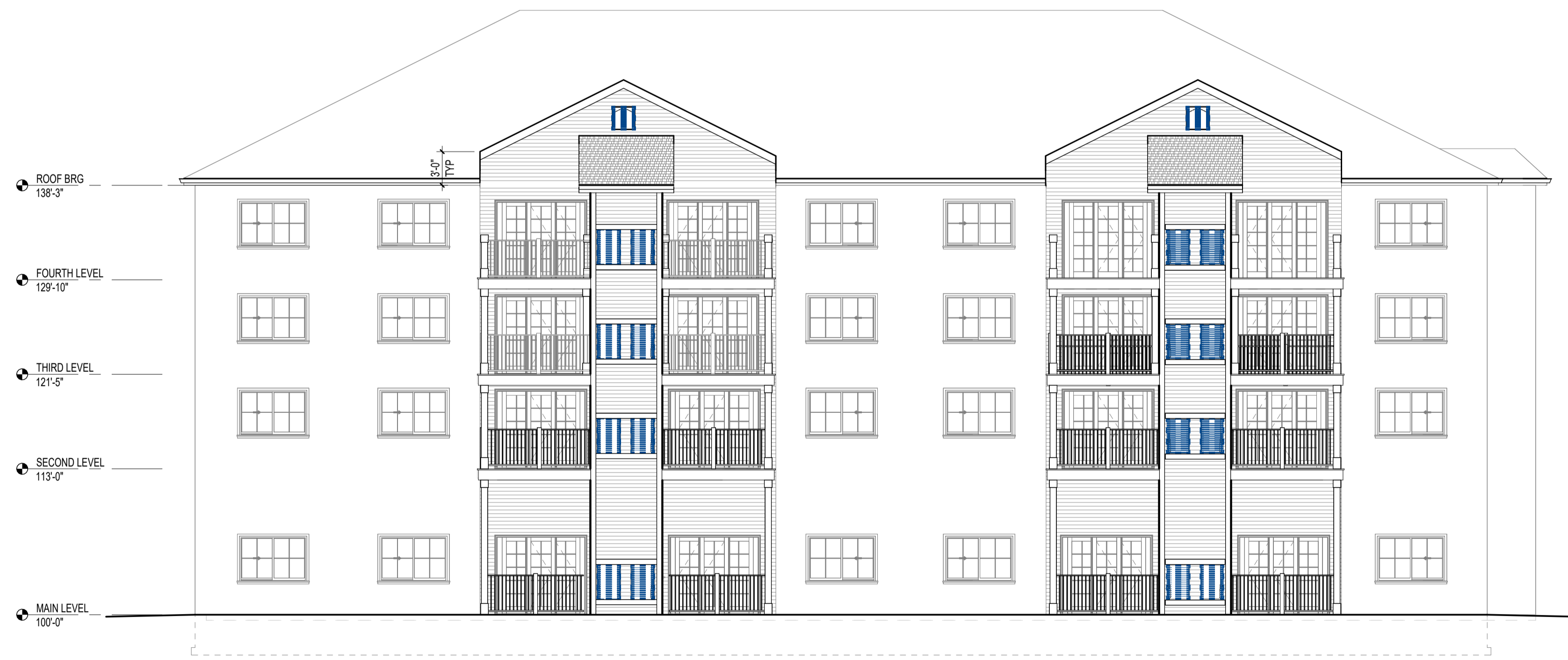
2 SOUTH ELEVATION WING "A" (STACK 1) A201 1/8" = 1'-0"
