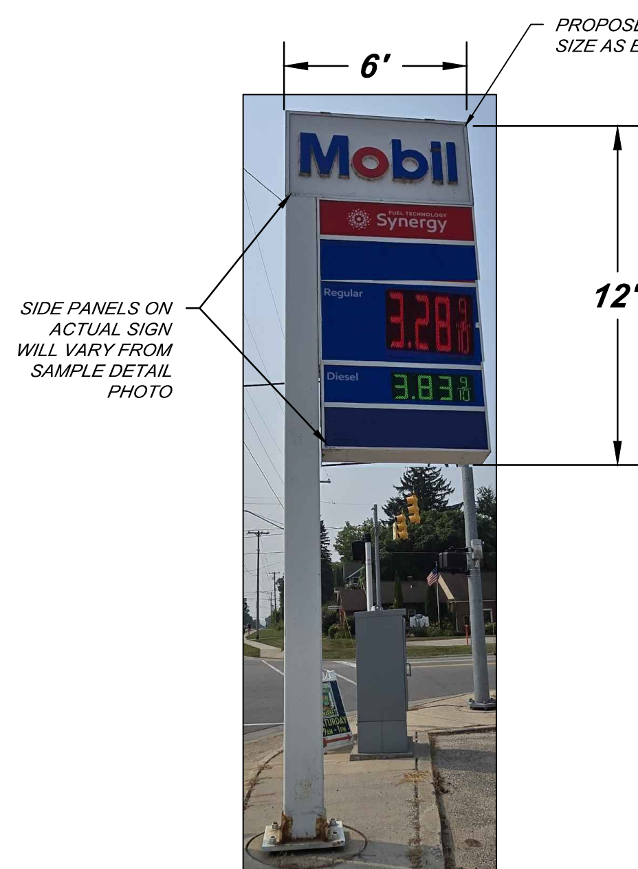
SAMPLE FREE STANDING GAS STATION SIGN DETAIL NOT TO SCALE
