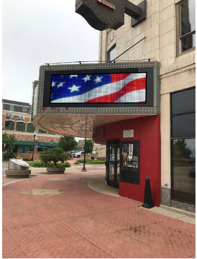
Existing exterior LED sign on marquee facing W. Western Avenue and matching the one facing 3 rd Street (left). Proposed 45"x147" exterior LED signs (active area 41.25"x144") will also match one another (right).
