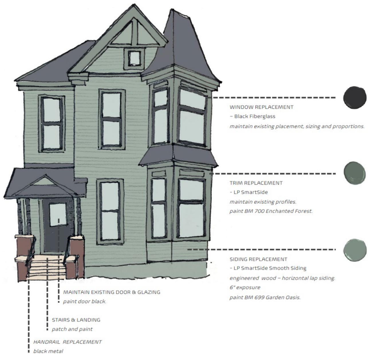
Rendered south elevation showing proposed changes.
