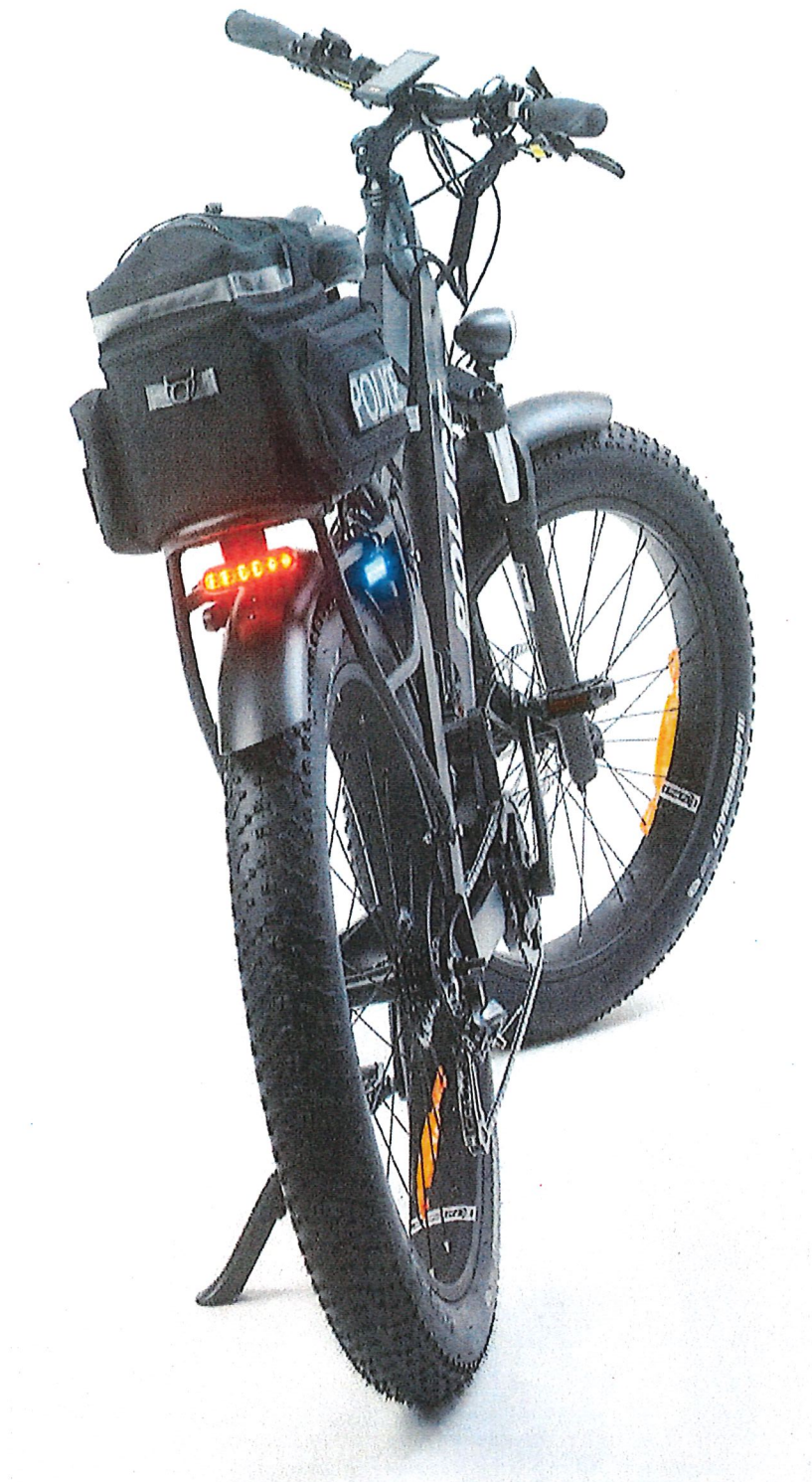
The RECON Police Interceptor is our flagship power bike, featuring state of the art technology. A best in class 1,000 watt mid driven, high torque, motor powered by a 48V/11.6 ah lithium ion battery and riding on 4" Fat Boy all terrain tires.
