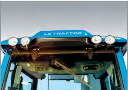
Rear work light Never be in the dark with this hands-free functional feature that allows light to be directed where you need it
