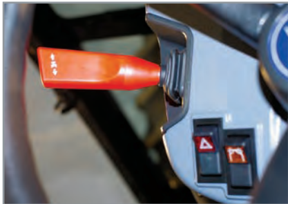
Power Shuttle Models Maximizes ease of use with effortless, clutch-less directional changes with the 40 forward / 40 reverse speeds with hi/Low mode
