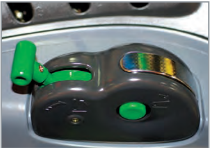
Position and draft control with Automatic lift Increases ease of use across a wider variety of implements
