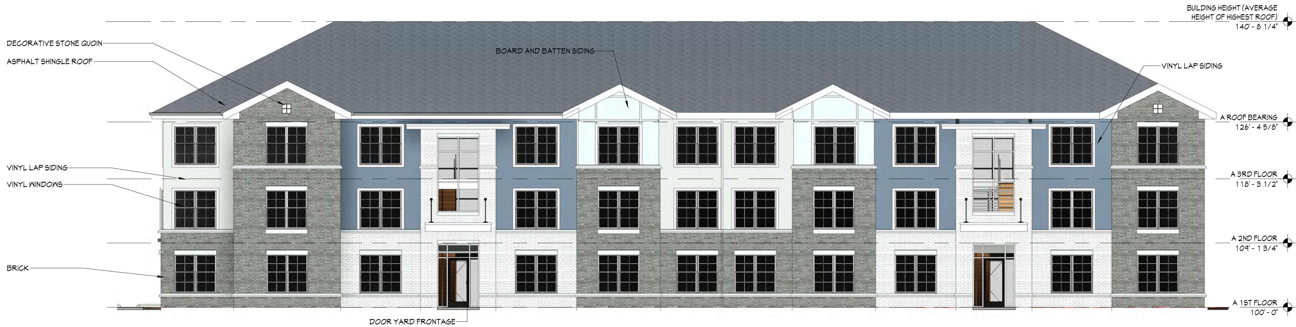
amity commons building B elevation 1/8" = 1'-0"
